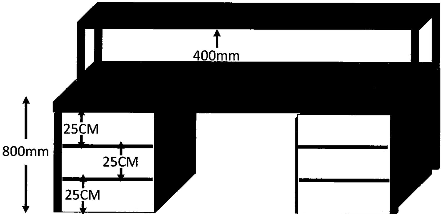
We included a raised platform at the end half of the table to accommodate decanting of water samples. We prefer Epoxy resin as the lab table top material for durability, chemical resistance, bacteria resistance, and easy-to-clean surface.
